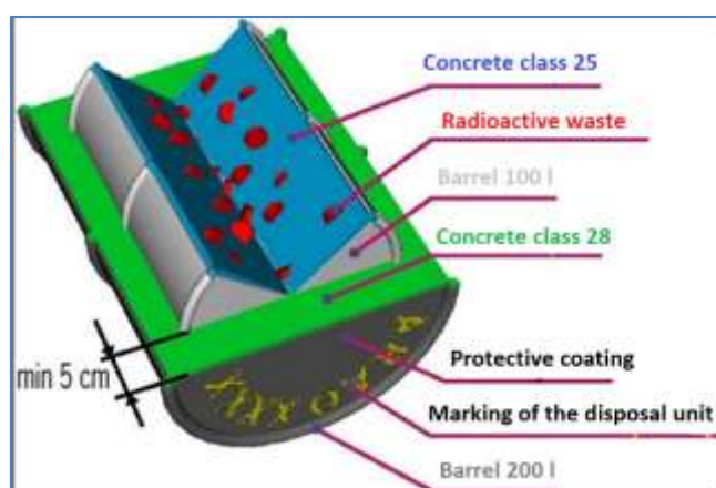
Figure 6: Radioactive waste disposal container – “sandwich” disposal unit (author: SÚRAO)
