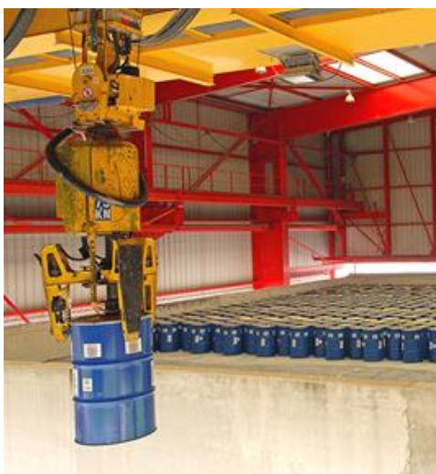
Figure 2-15 Metallic waste packages in vault
