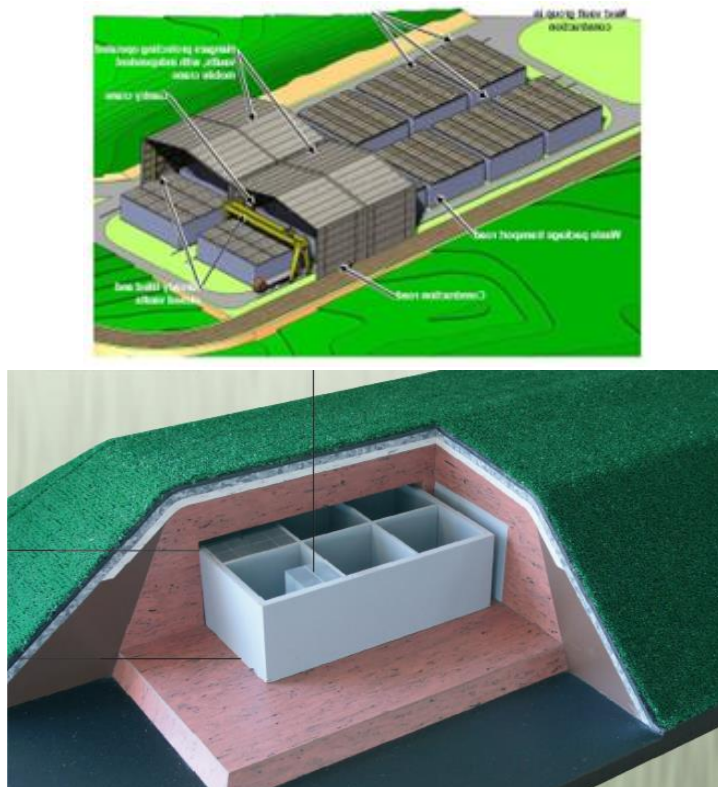
Figure 2-18 Conceptual model of NSR at Stabatiškė site: top – during operation, Bottom – closure
