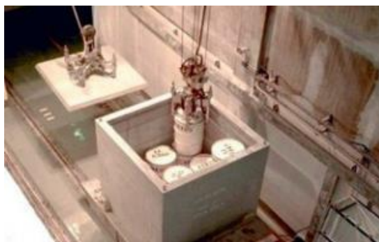
Figure 2-34 Packages into a disposal unit
