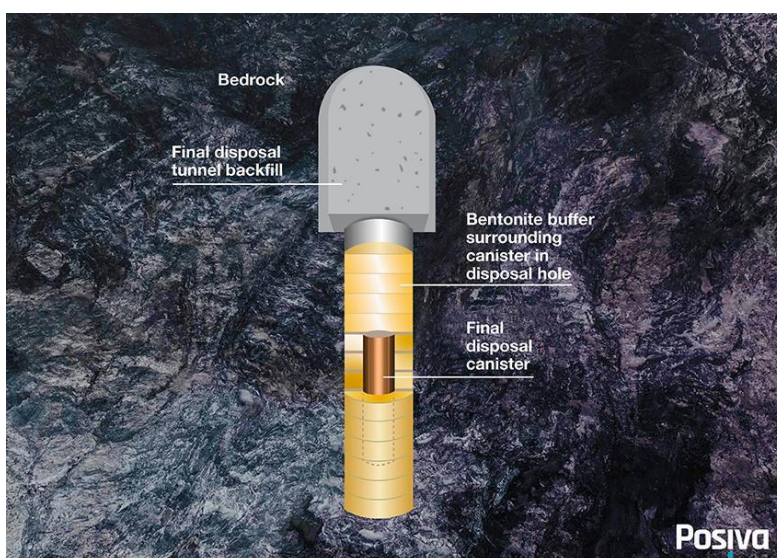
Figure 3 A canister in a deposition hole
