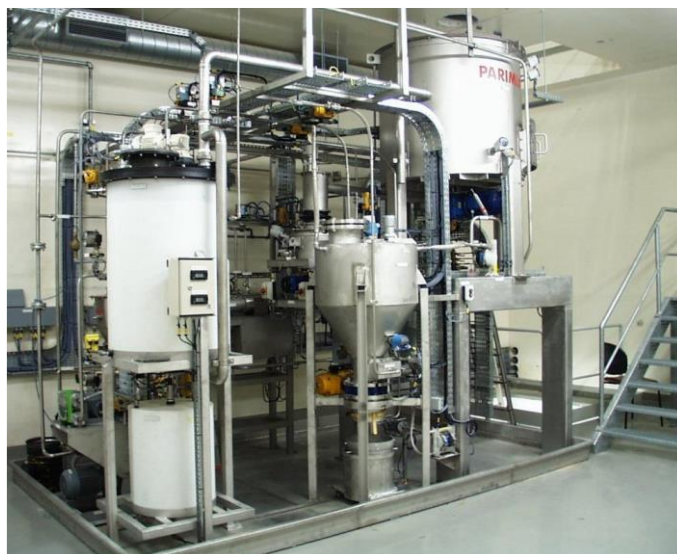
Figure 6 - View of the off-gas system of the incinerator. (Courtesy of Belgoprocess).
