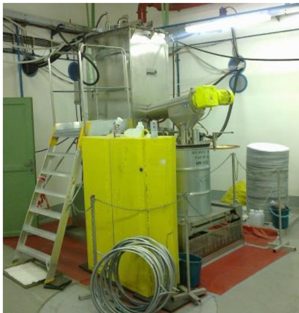
Figure 9 - On-site unit to condition ion exchange resin using SIAL® geopolymer at Dukovany NPP, Czech Republic (Courtesy of Jacobs).
