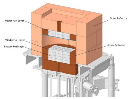
Lead plutonium measurements, visualization of the full assembly
