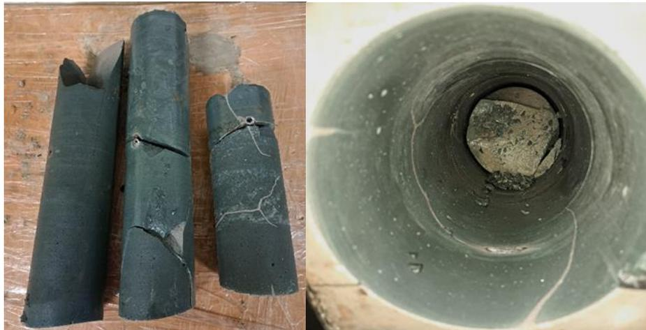
**Figure 163** Samples extracted from the bottom, centre and top of the drum (left) and a close-up photo of the drilled hole in the drum (right)
