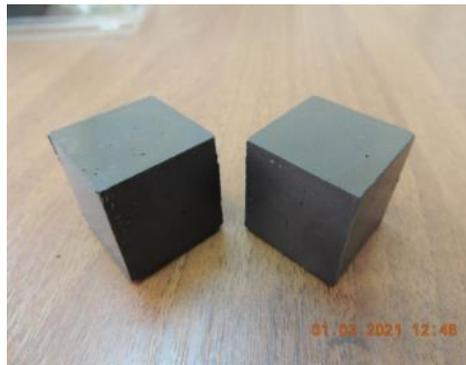
**Figure 6** Geopolymer samples with 30% of Shellspirax oil
