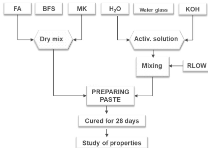
**Figure 100** Sample production process by KIPT
