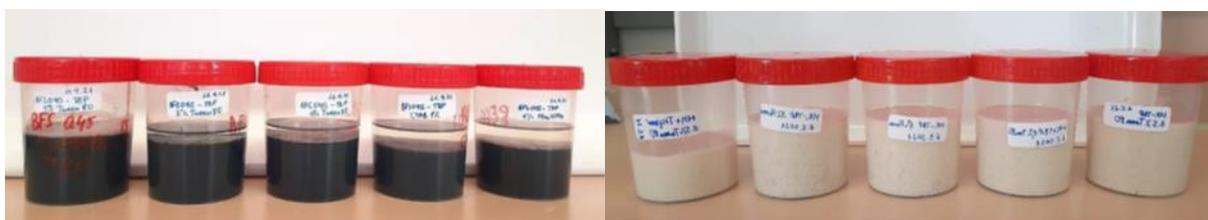
**Figure 35** State of waste-forms with AAS (left) and with MK-based geopolymer (right) when using Tween 80 as a surfactant after 7 days of curing
