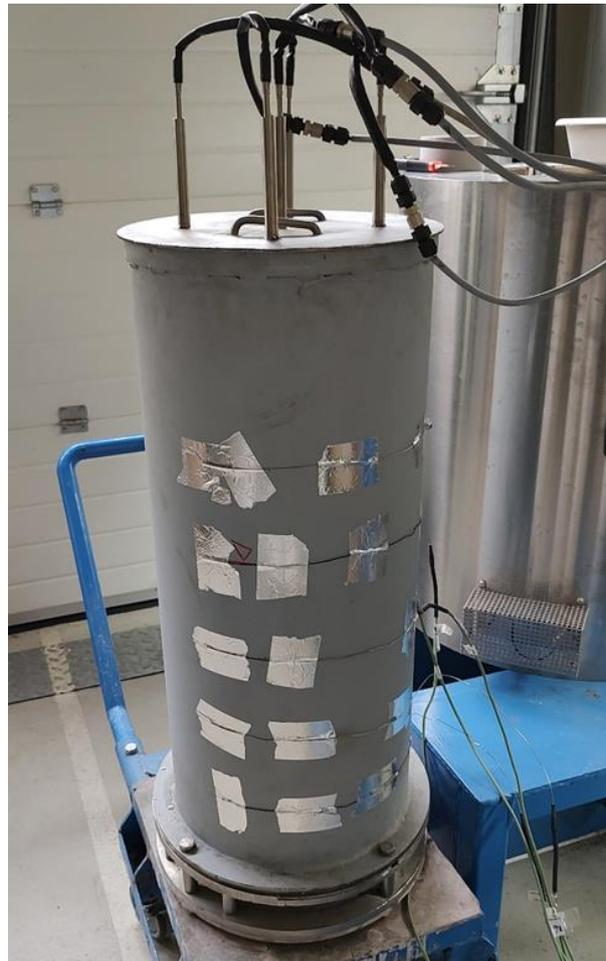
**Figure 151** Thermocouple layout on the lid (left) and on the surface of the 50 L drum (right)
