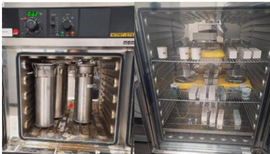
Figure 25 ASR test (left) and carbonation test (right)
