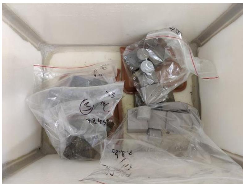
**Figure 125** Curing of the samples in a closed box with the addition of water
