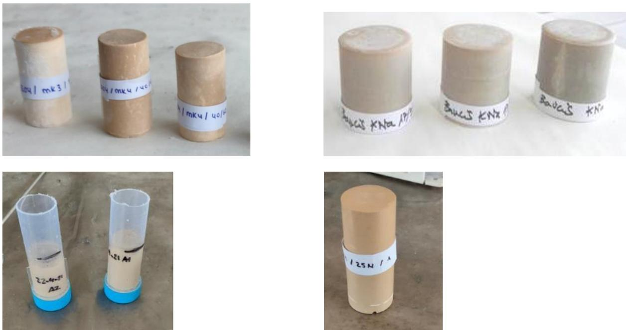
**Figure 1** Geopolymer samples
