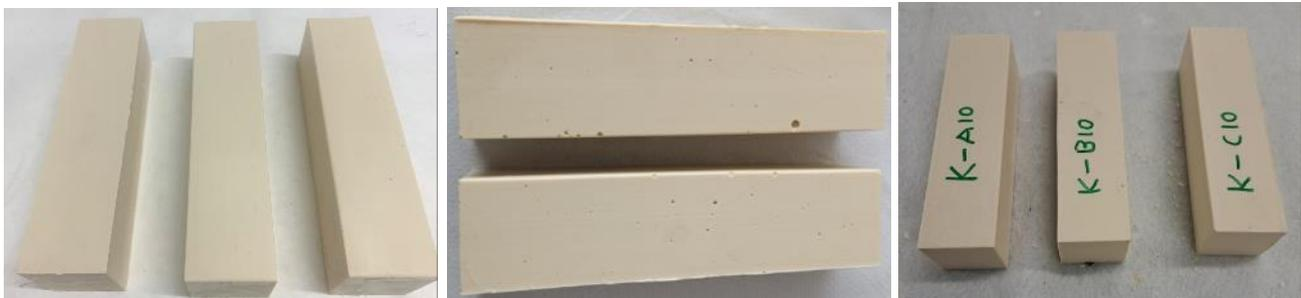
**Figure 41** Hardened samples of Geopolymer without RLOW surrogate (left), with 30% vol. of oil surrogate (middle) and 10-30% vol. of scintillation cocktail surrogate (right)
