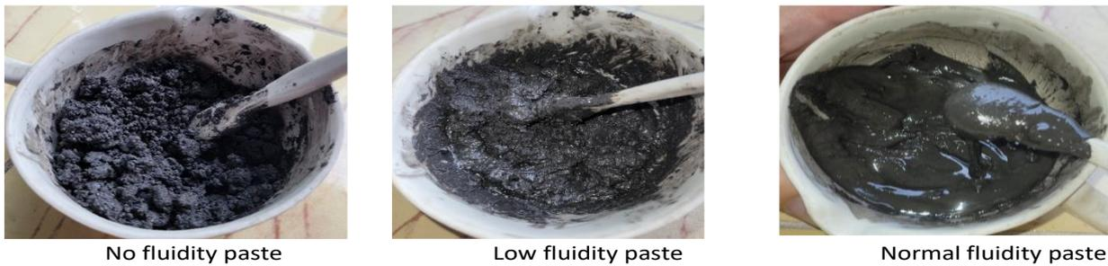
**Figure 95** No fluidity paste (left), low fluidity paste (middle) and normal fluidity paste (right)
