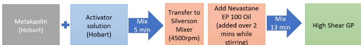
**Figure 56** Mixing methods used to prepare samples containing Nevastane oil
