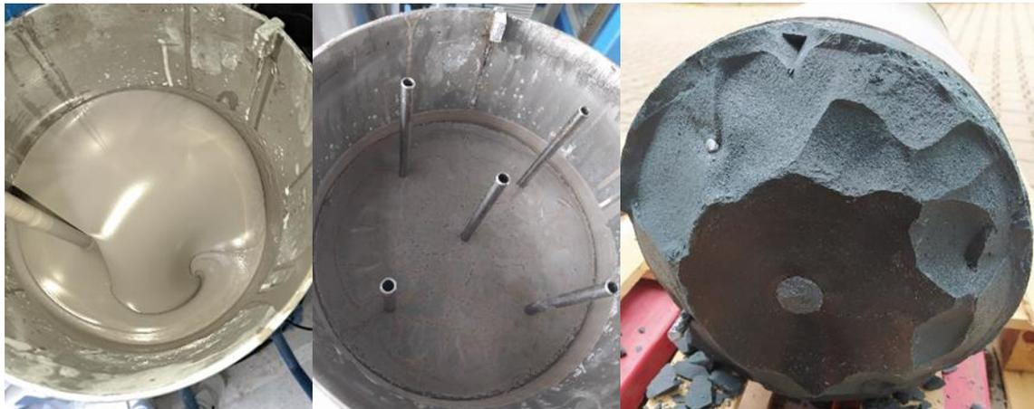
**Figure 157** Geopolymer composition during mixing (left), after curing (middle) and cut bottom of the drum after curing (right)
