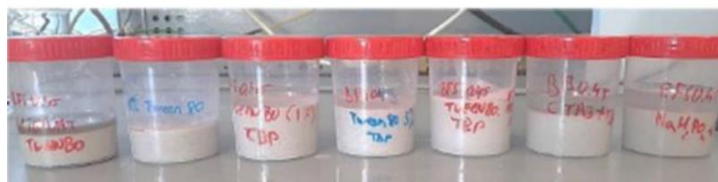
**Figure 32** Fresh mixtures containing AAS and wastes (TBP, ionic liquids), using different surfactants
