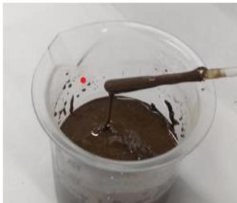
**Figure 13** Fresh geopolymeric grout
