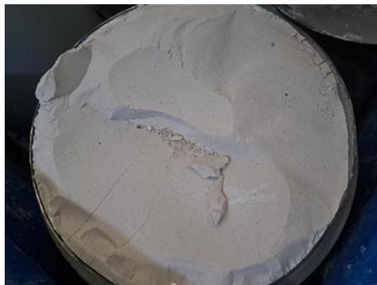
**Figure 156** Geopolymer composition at the bottom of the drum after curing
