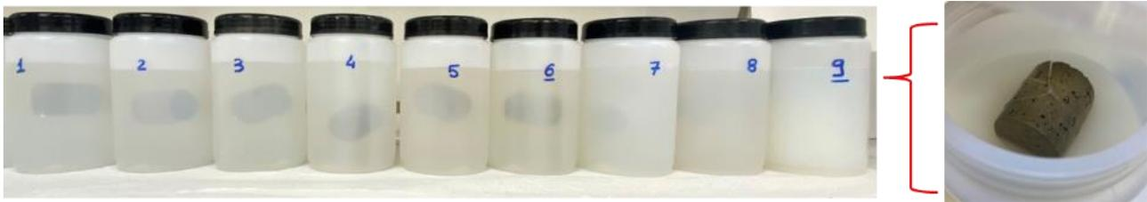
**Figure 119** On the left - samples used to study the effect of rPU and RLOW loading on immersion stability, on the right - a sample surrounded by leachant of a milky consistency.
