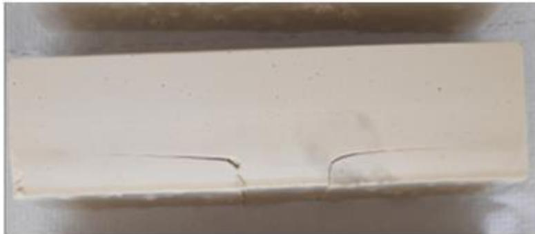
**Figure 40** Cracks in the surface of the geopolymer samples
