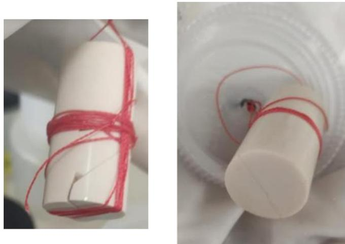
**Figure 48** Samples of geopolymers with InstaGel Plus after leaching test
