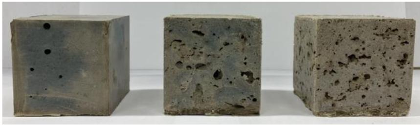
**Figure 117** Samples with different rPU loading (no RLOW): left – 0 wt.%, middle – 5 wt.%, right 10 wt.%
