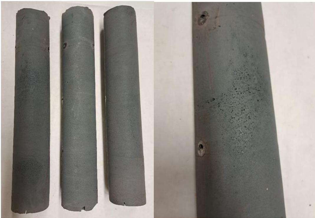
**Figure 170** Samples extracted from the top, centre and bottom of the drum (left) and a close-up photo of the pores in the top sample (right)
