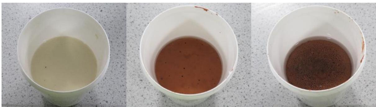
**Figure 38** 20 vol% loading of TBP in Metamax® geopolymer (left), 10 vol% loading of TBP in Argicem® geopolymer (centre) and 20 vol% loading of TBP in Argicem® geopolymer (right).
