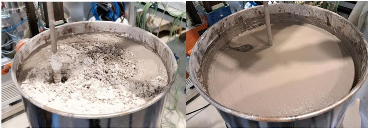
**Figure 159** Geopolymer mixing
