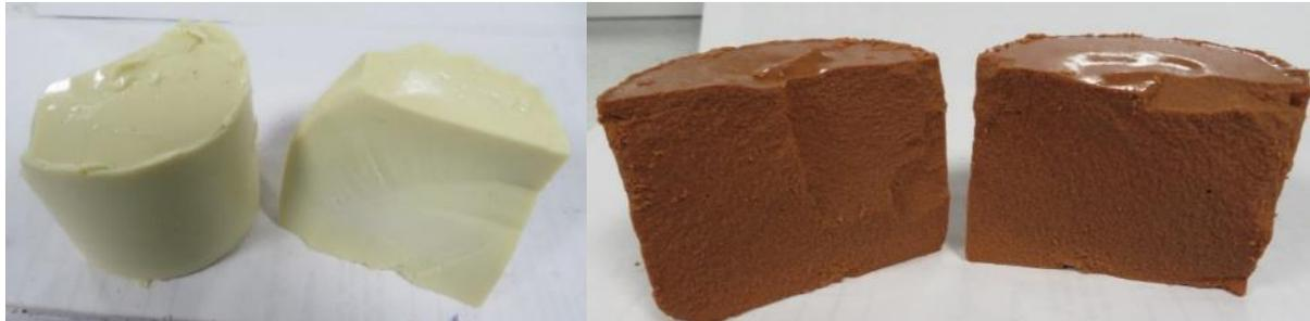
**Figure 37** 50 vol% loading of Nevastane EP 100 in Metamax® geopolymer (left) and Argicem® geopolymer (right)
