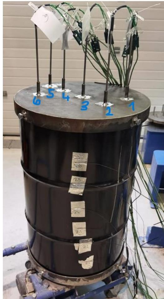
**Figure 152** Thermocouple layout on the lid (left) and on the surface of the 100 L drum (right)
