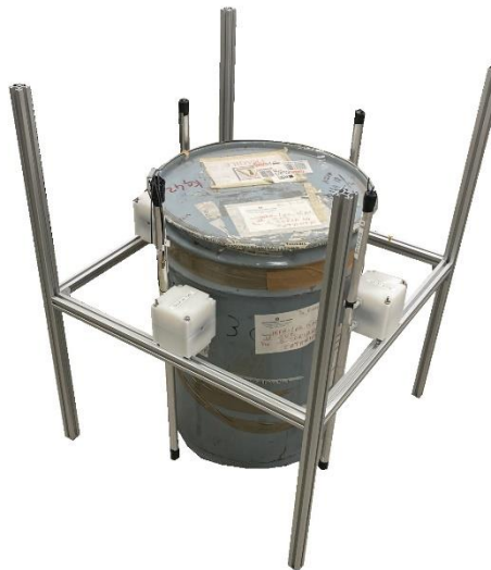
Figure 22. The lightweight aluminum frame to support the SiLiF and SciFi sensors around the mock-up drum, assembled using modular Bosch Rexroth profiles.
