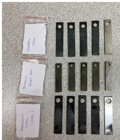
Figure 2: The picture of the oxidised – and pristine samples.
