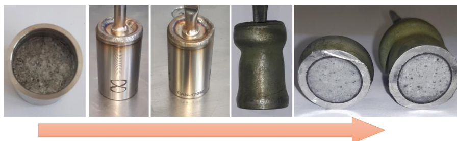
Figure 1. HIP treatment of IRIS ashes at USFD from left to right: can packing, welding, crimping, thermal treatment (1250 °C), and sectioning open the can.
