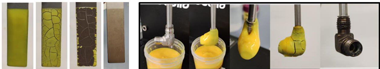
Figure 4: Corrosion of a stainless steel plan coupon by gel deposition (left) and a stainless steel complex geometry item using a bath of gel (right).
