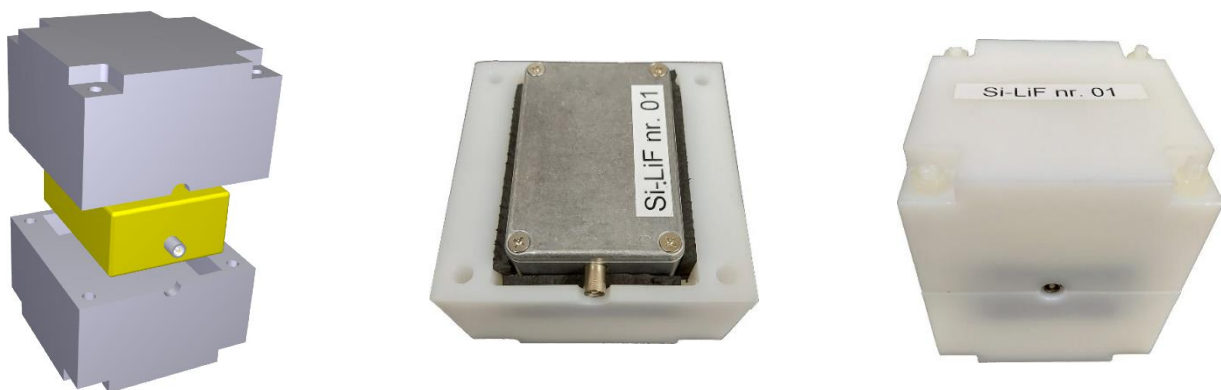
Figure 18. Left: sketch of the SiLiF detector (in yellow) and its arrangement inside the moderator (in grey). Center: a SiLiF hosted in a half moderator. Right: final assembly of a SiLiF.
