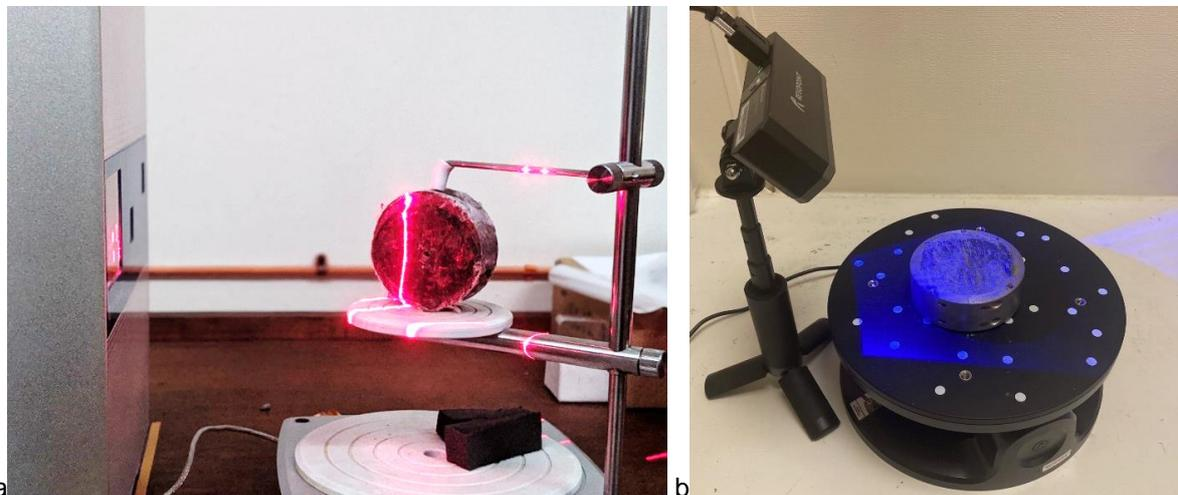
Figure 8 - Laser scanning of fracture surfaces. a) NextEngine 3D Scanner HD; b) Revopoint MINI 3D Scanner.
