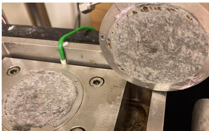
Figure 17 - Photograph of the fracture surface formed after repeat shearing.
