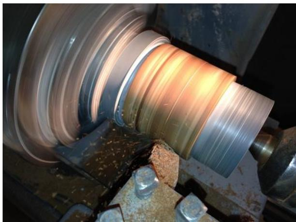
Figure 1 - Callovo-Oxfordian Claystone sample being cut on a lathe during the careful sample preparation process.
