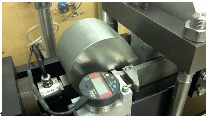
Figure 3 - Components of the Heated Shear Rig. a) Photo of the complete apparatus; b) Loading frame with normal load cells at the bottom; c) normal load ram (yellow); d) sample assembly, shear load cell and horizontal displacement sensor.
