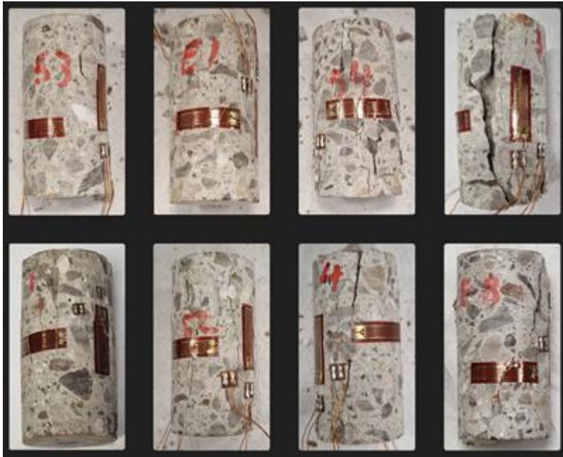
Figure 3-4 Examples of samples after failure in uniaxial compression.
