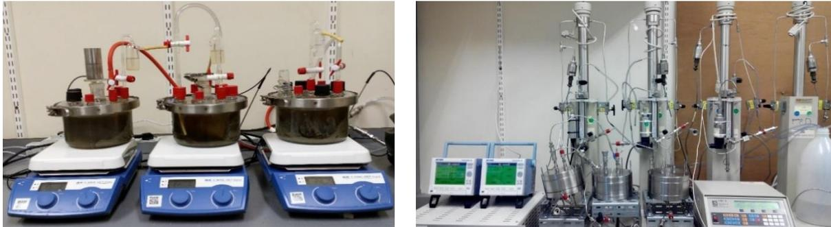
Figure 2-16 Test setups for batch (left) and percolation (right) experiment
