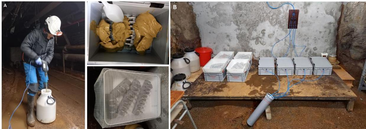
Figure 2-18 A) Preparation of the in-situ experiment at URF Bukov. B) Arrangement of the experimental setups for studying interactions of LPC samples under in-situ conditions (air, groundwater, bentonite suspension)
