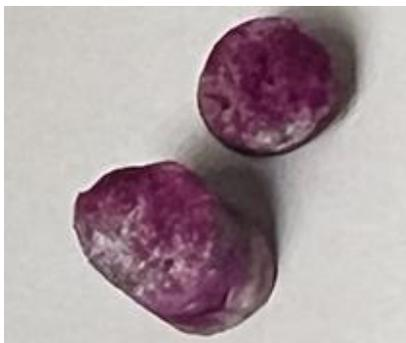
*Figure 2-4 Non-carbonated surface detected on mortar specimen after pre-drying at 20 °C / 65 % HR and 5 days of accelerated carbonation (diameter of the specimens is 4 mm)*
