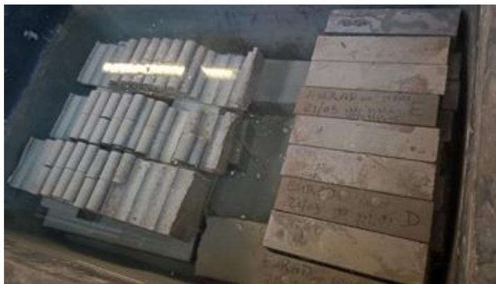
Figure 2-1 Curing of cored cylindrical samples (on the left) and prismatic beams for 3-point bending test
