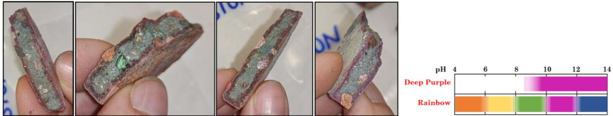
Figure 4-30 pH determination of LPC\_SURAO by rainbow indicator (T3 – 18 months aged samples; broken discs after punch tests).
