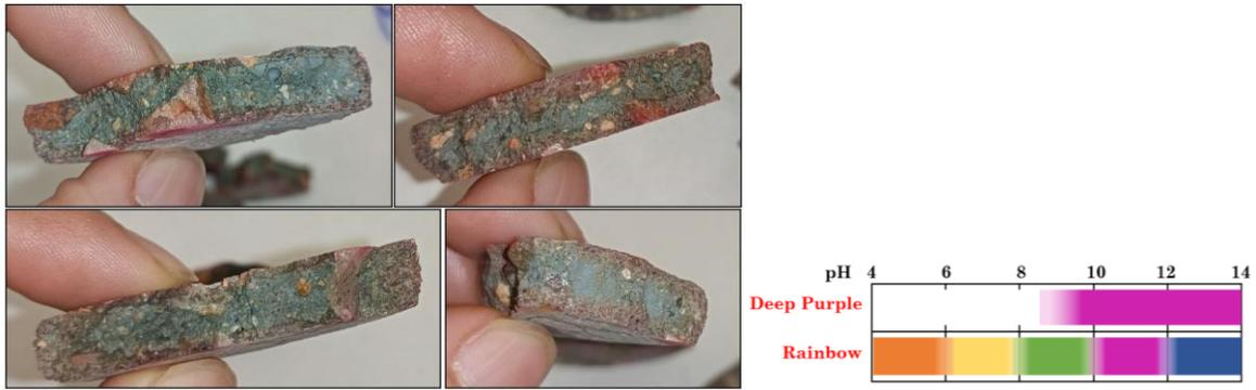
Figure 4-19 pH determination of LPC\_SURAO by rainbow indicator (T3 – 18 months aged samples; broken discs after punch tests).
