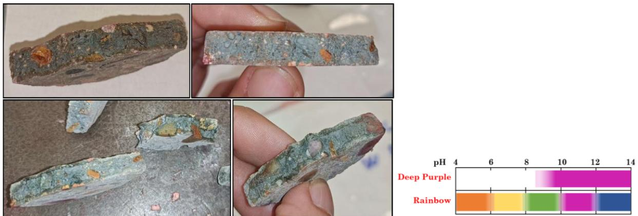
Figure 4-25 pH determination of LPC\_SURAO by rainbow indicator (T3 – 18 months aged samples; broken discs after punch tests).
