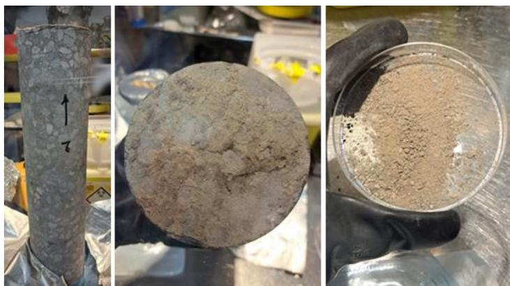
Figure 4-13 Overview of the complete concrete core (left); the concrete-clay interface (middle) and the clay on the concrete core (right)
