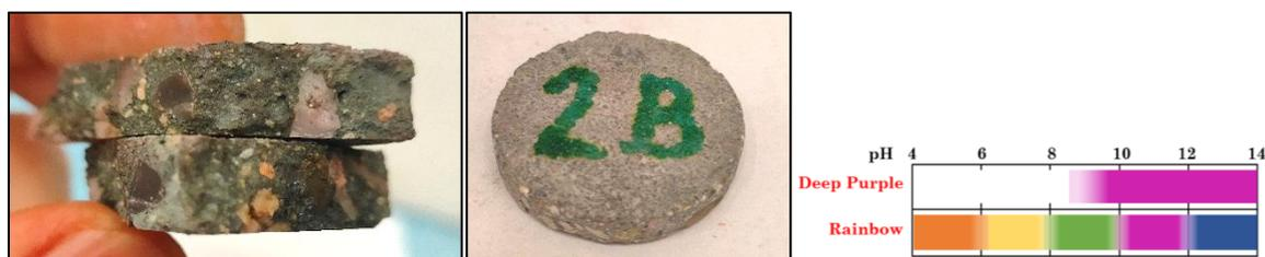
Figure 5-25 pH visualisation by rainbow indicator - cube cut edge (surface exposed to air for 3 years URL Bukov at 100% RH + 2 years at CTU lab with 30-50% RH).
