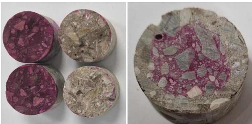
Figure 3-3 Sound and 100% + carbonated samples (left), sample at an intermediate state of carbonation (50 % carbonation state, right figure).
