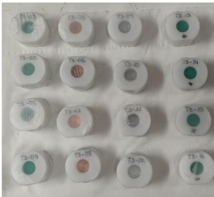
Figure 52 – Picture of sixteen closed cells installed with copper and carbon steel metal coupons, or magnetite oxide, placed over one surface of compacted bentonite samples, at different conditions (*Table 22*) prepared for gamma radiation experiments under aerobic conditions.
