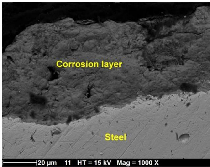
Figure 24 SEM photo of steel hydrated at 76% RH (side facing the atmosphere) for 14 days in the experiment with bentonite (Sample F58).
