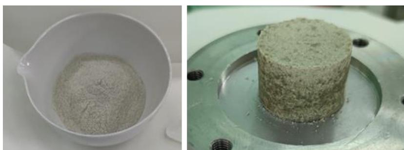
Figure 48 – (a) Powder FEBEX bentonite grounded and sieved to a fraction < 0.5 mm. (b) Example of compacted bentonite sample hydrated with porewater at desired saturation degree.
