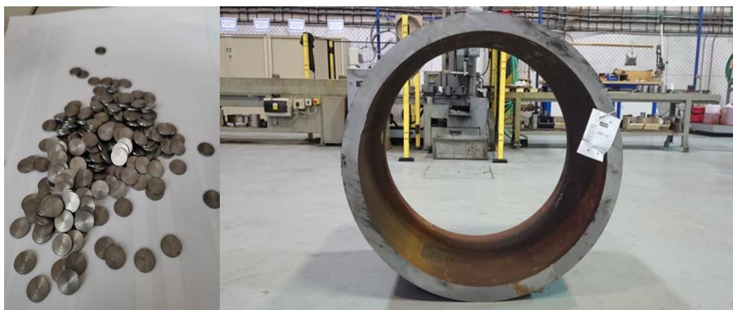
Figure 28 Left – carbon steel disks, right – outer case of the canister in the Czech concept.
