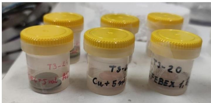
Figure 50 – Samples of different metal coupons immersed in 5 mL of different bentonite porewater (PW-1.4, PW-1.6, composition in Table 8) or deionised water (DW) prepared in isotactic polypropylene tubes.
