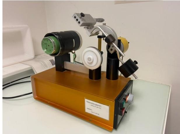
Figure 2 Diamond Wire Saw.
