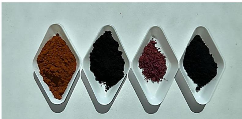
Figure 47 – Selected corrosion products. From Left to Right:  $Fe_2O_3$ ,  $Fe_3O_4$ ,  $Cu_2O$  and  $CuO$  commercial nano-powder oxides.
