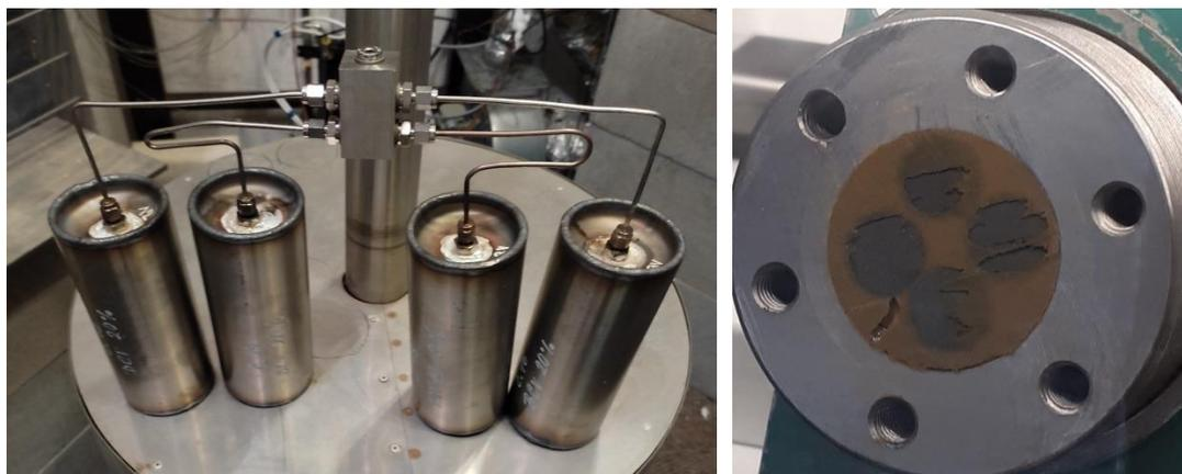
Figure 30 Left – steel vessels containing steel cells connected by metal capillaries with saturation medium situated in the irradiation area, right - steel cell containing compacted BCV bentonite and carbon steel coupons during disassembly (cell no. 22).
