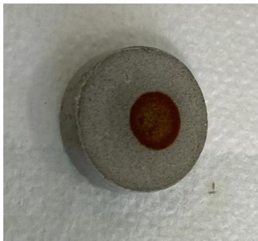
Figure 18 Corrosion layer transported in clay from unirradiated sample F25
