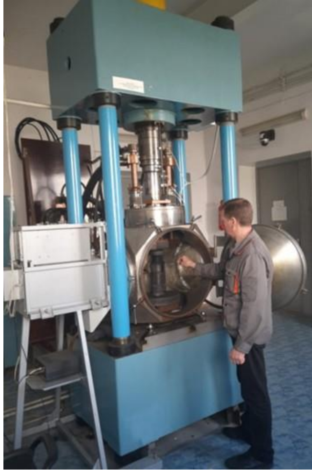
Figure 27. Laboratory HP facility for sintering ceramic materials.
