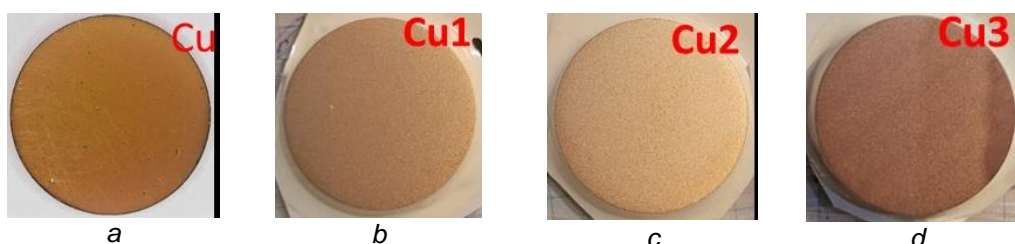
Figure 71. Photos of the steel samples with deposited metallic Cu coatings with thickness up to 30 \mu\text{m} under different parameters of the deposition processes by MS (a) and CAE (b, c, d)
