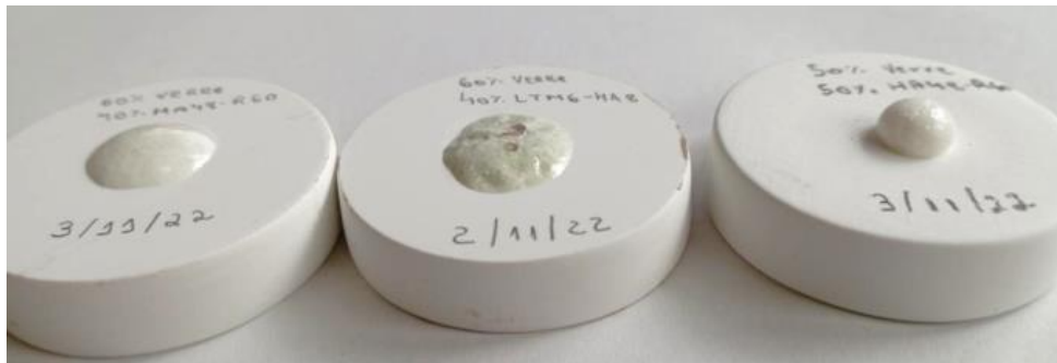
Figure 13. Wetting test of composite materials. The left sample is composed of 60% glass-40 % SiO 2 -AlO 2 blend, the middle sample is composed of 60% glass-40 % SiO 2 -AlO 2 -Bi 2 O 3 -CuO with nano SiC blend, and the right sample is composed of 50% glass-50 % SiO 2 -AlO 2 blend.
