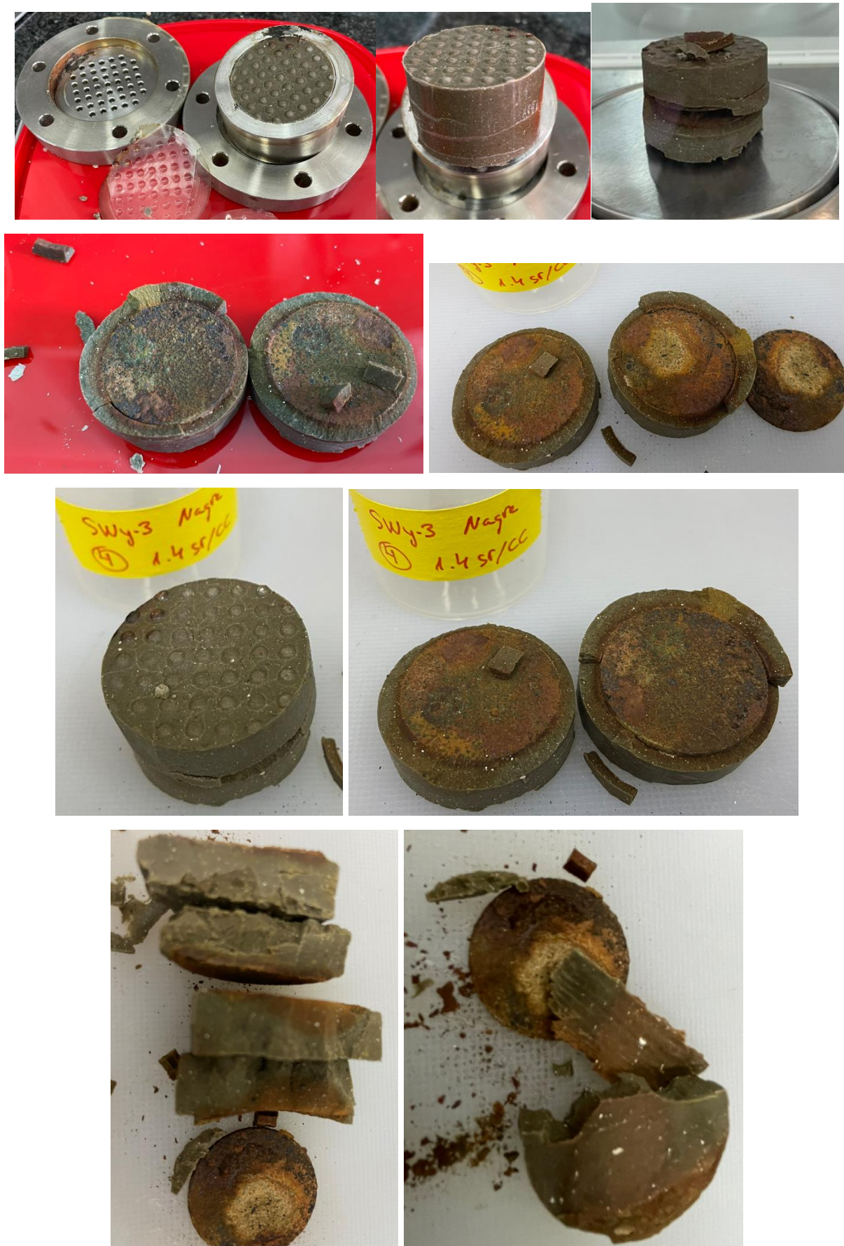
Figure 18 – Dismantling of the SWy3 bentonite compacted at 1.4 g/cm 3 with Nagra carbon steel coupon showing the alteration of the bentonite and the corroded coupon.
