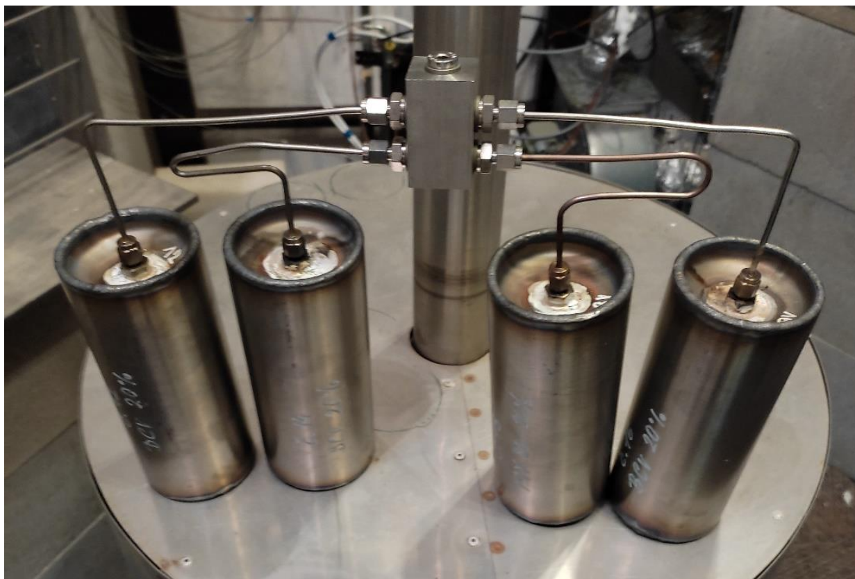
Figure 108 – Steel vessels containing steel modules connected by metal capillaries with saturation medium situated in the irradiation area.
