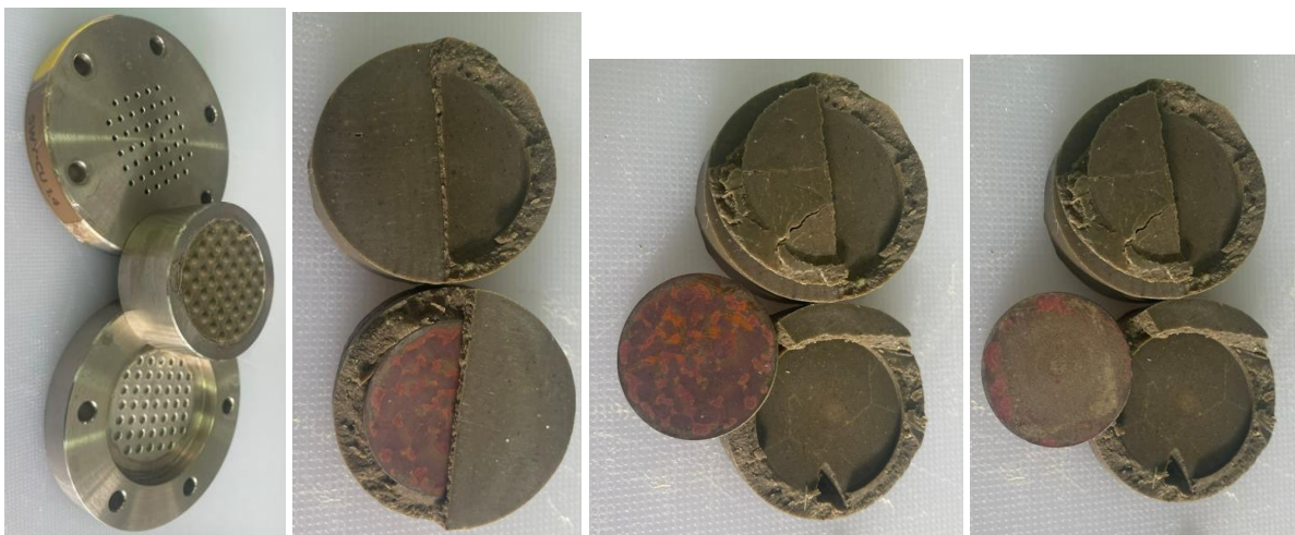
Figure 49 – Dismantling of the SWy-3 bentonite compacted at 1.4 \text{ g/cm}^3 with SKB Cu-OFP coupon.
