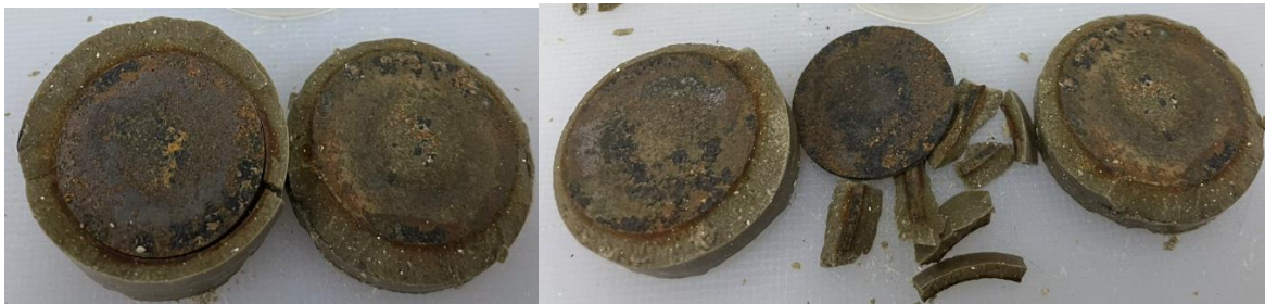
Figure 19 – Dismantling of the SWy3 bentonite compacted at 1.6 \text{ g/cm}^3 with Nagra carbon steel coupon showing the corroded coupon and the compacted bentonite.
