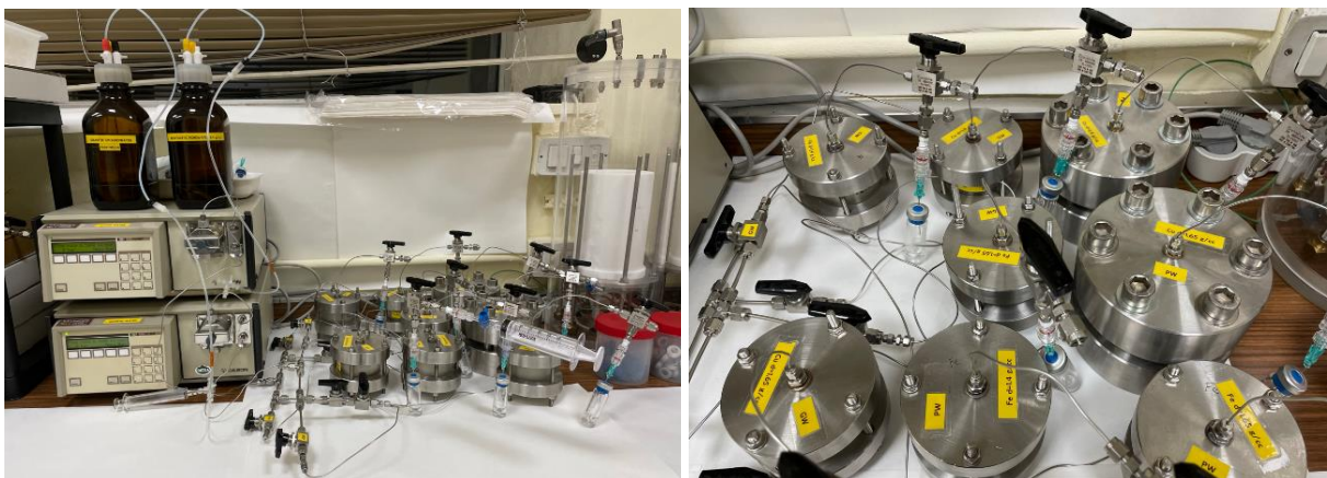
Figure 5 – Setup of the infiltration cells used for dynamic experiments.
