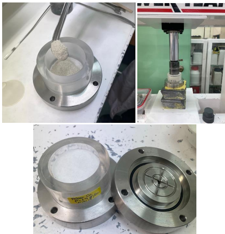
Figure 6 – Detail of the preparation of the compacted cells for infiltration experiments.
