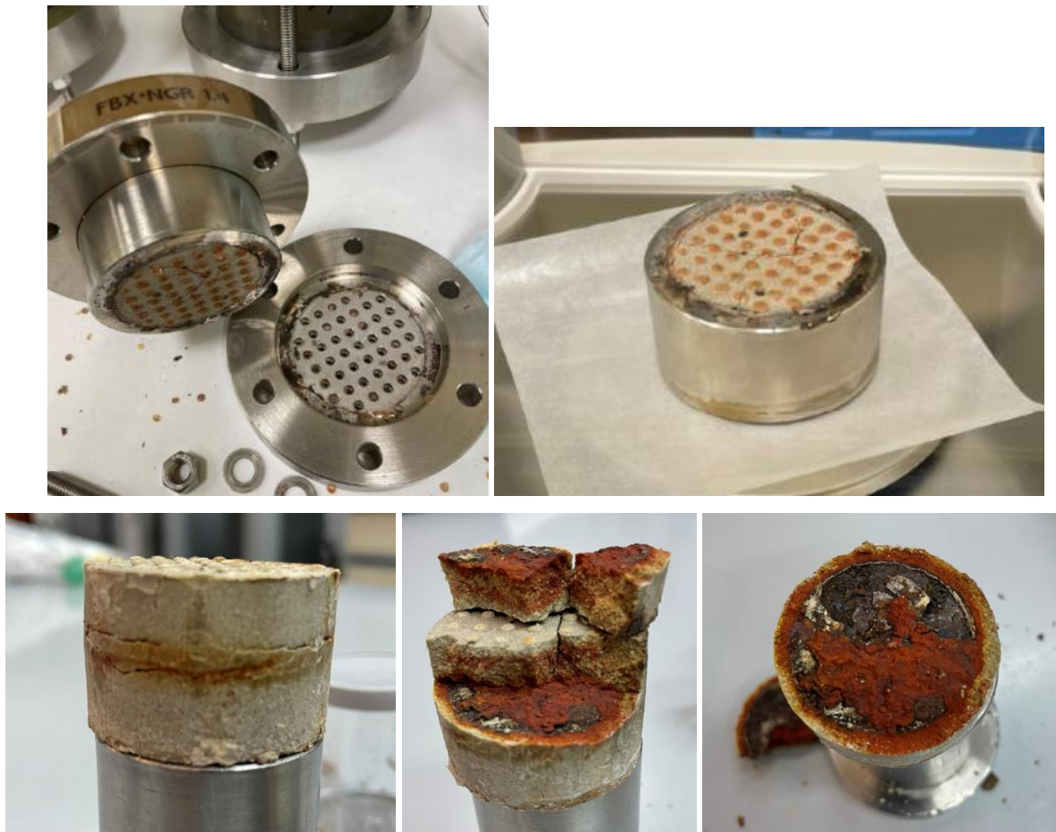
Figure 16 – Dismantling of the FEBEX bentonite compacted at 1.4 g/cm 3 with Nagra carbon steel coupon: altered bentonite and corroded corrosion is shown.
