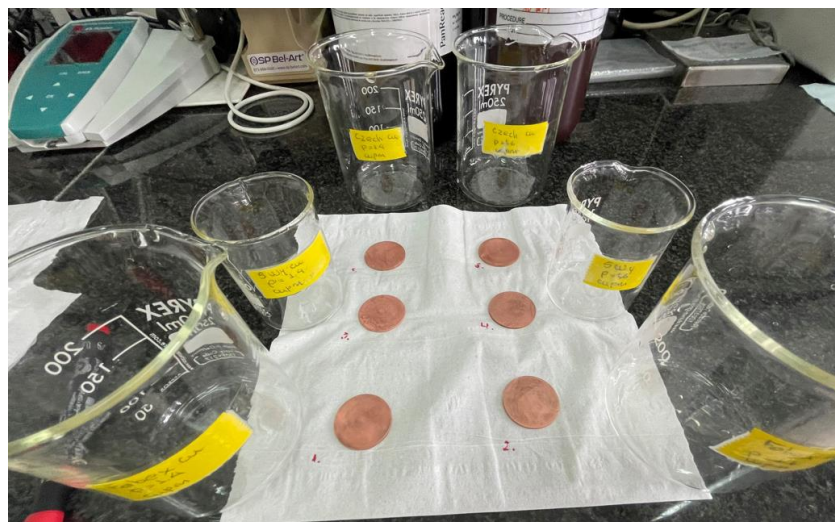
Figure 54 – Visual aspect of the corroded Cu-coupons after the five washings prior to determining corrosion rate.
