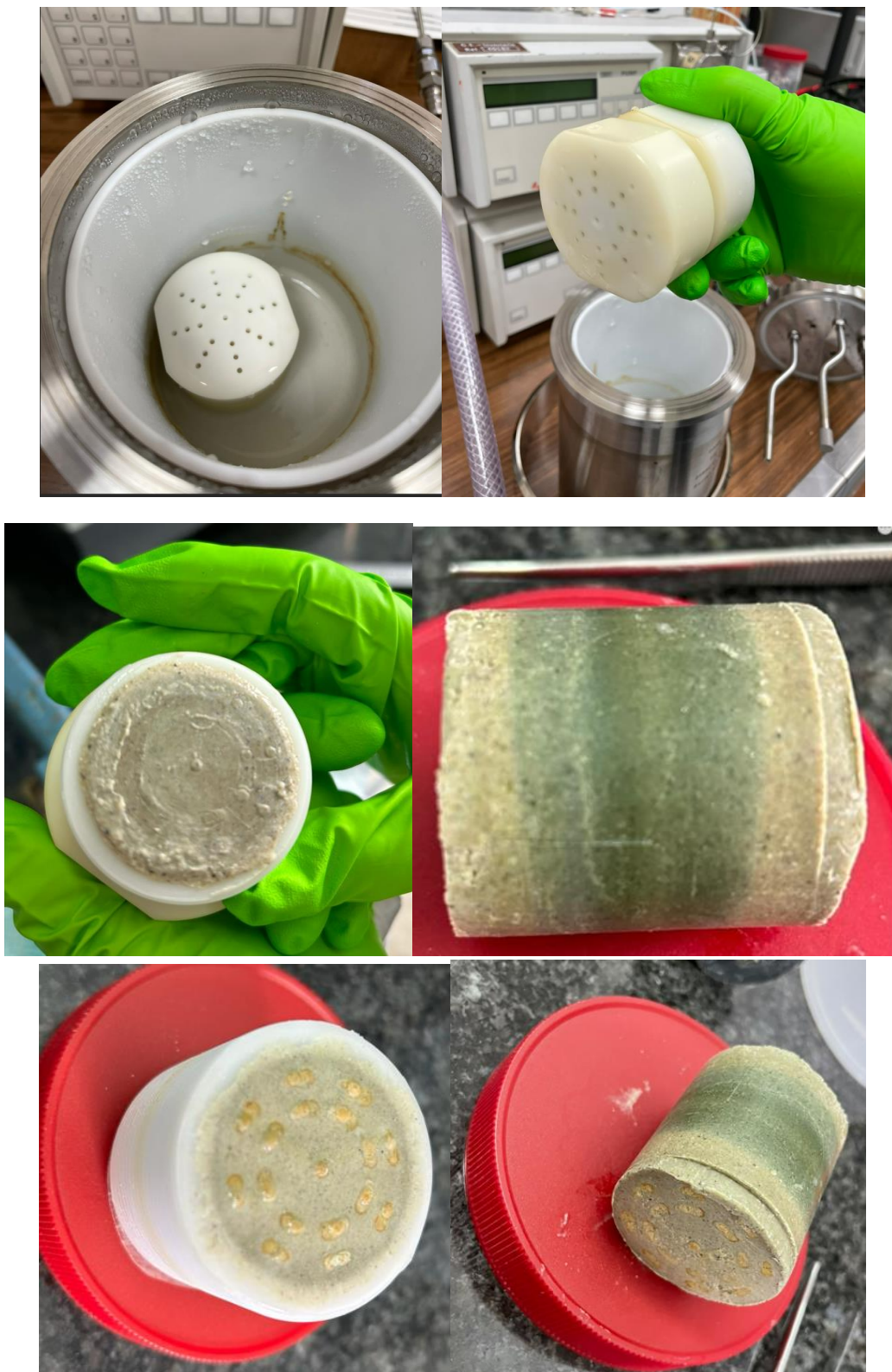
Figure 75 – Detail of sampling of bentonite at the end of the static experiment in the reactor at 80°C: FEBEX bentonite at 1.4 g/cm 3 of dry density.
