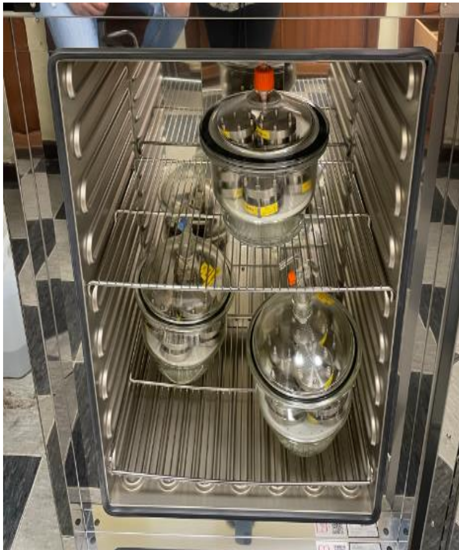
Figure 10 – Experimental setup for convective water-vapor fluxes at 80 .
