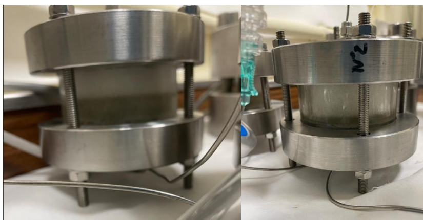
Figure 14 – Detail of the degree of saturation of the bentonite: a) compacted at 1.4 g/cm 3 , and b) compacted at 1.65 g/cm 3 .
