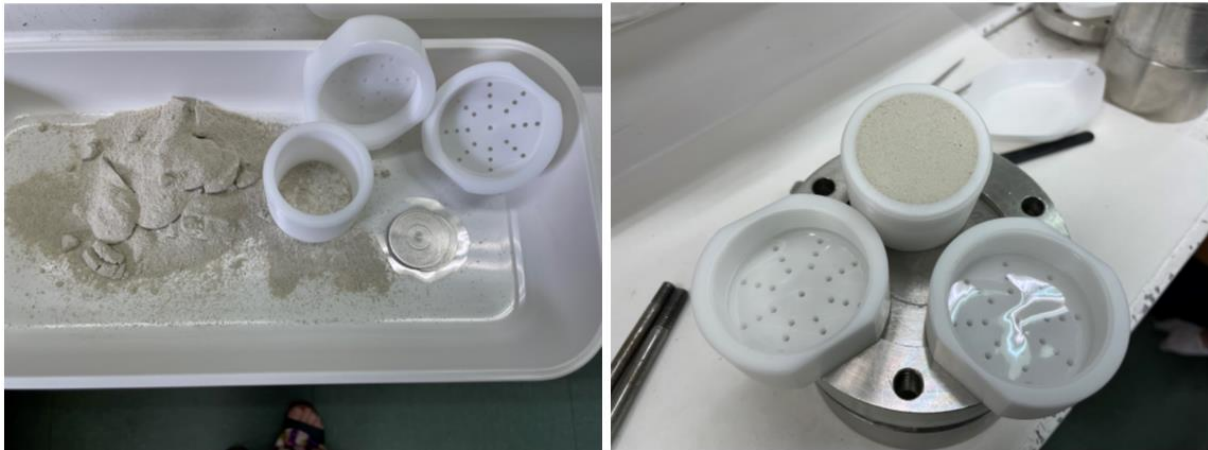
Figure 11 – Detail of the bentonite, Nagra C-steel coupon and cell used for static experiments.
