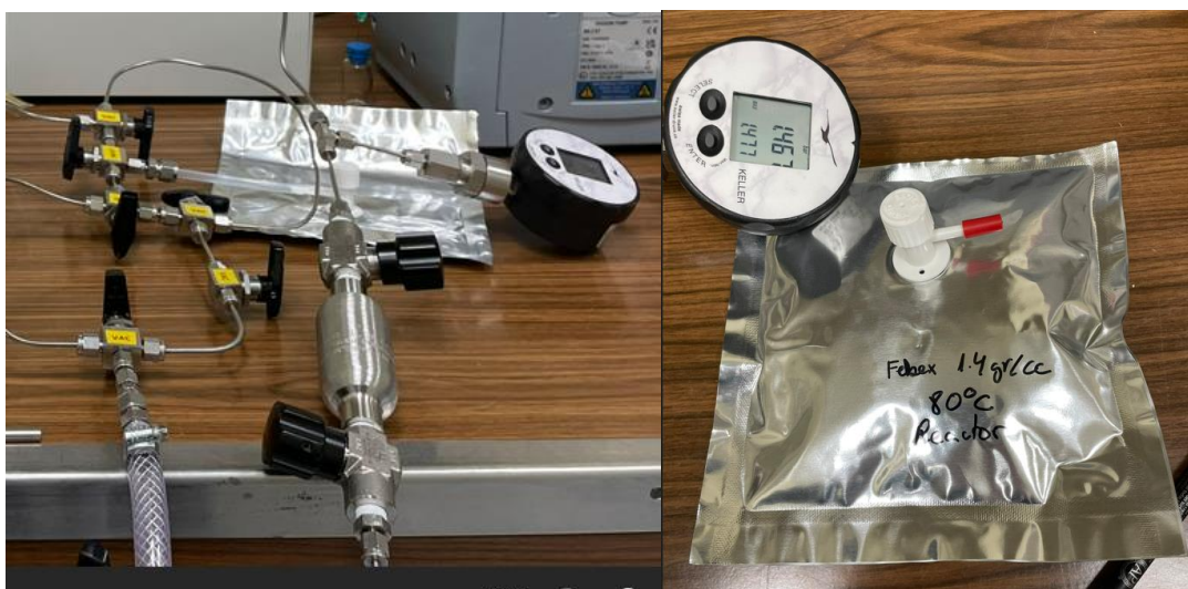
Figure 13 – Collection of gas and water samples at the end of the static experiment in the reactor at 80 °C: FEBEX bentonite at 1.4 g/cm 3 of dry density.
