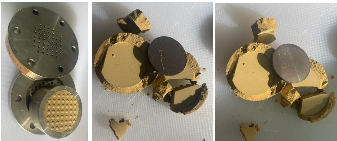
Figure 51 – Dismantling of the Czech bentonite compacted at 1.4 g/cm 3 with SKB Cu-OFP coupon.
