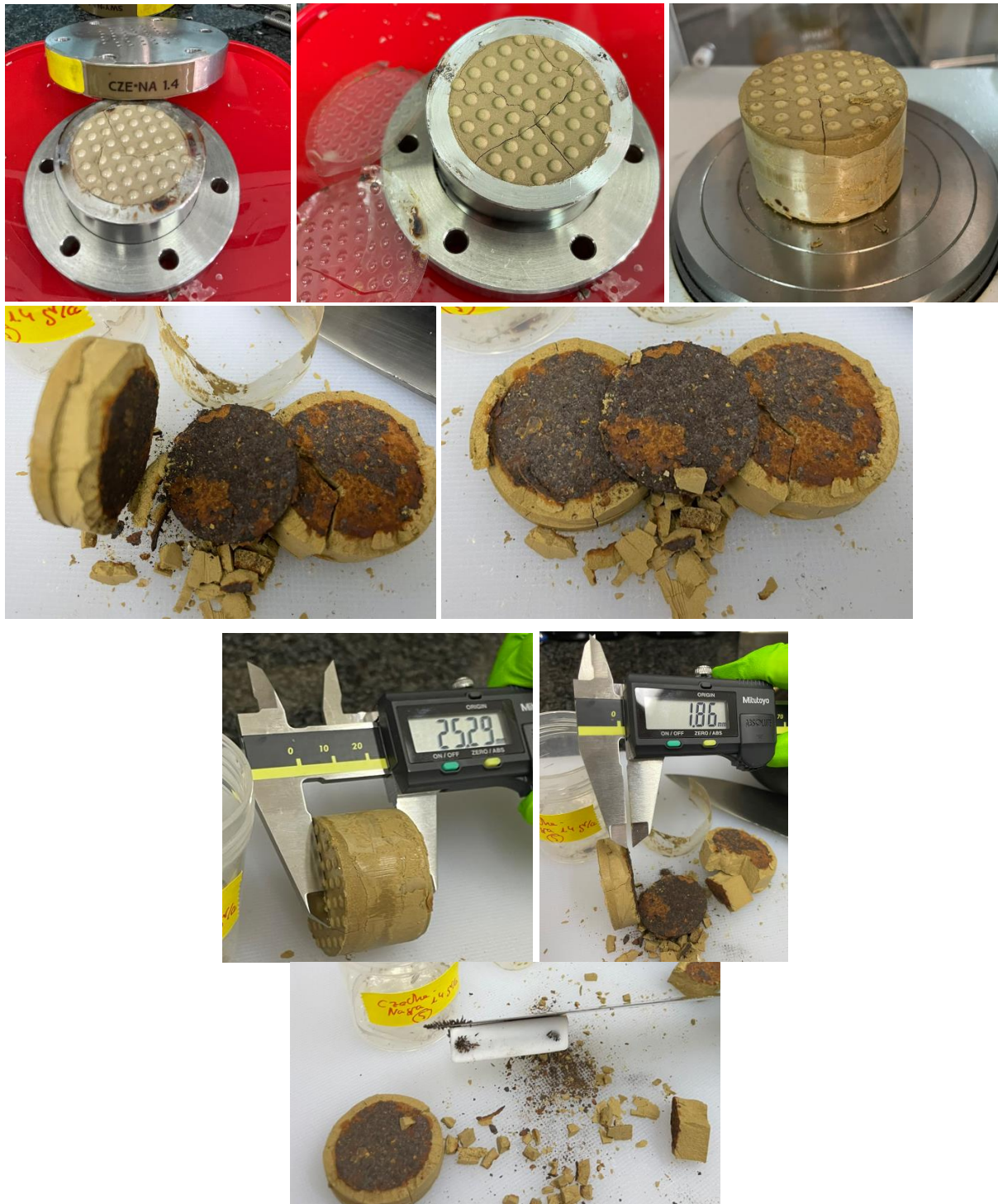
Figure 21 – Dismantling of the Czech bentonite compacted at 1.4 g/cm 3 with Nagra carbon steel coupon showing the alteration of the bentonite and the corroded coupon.
