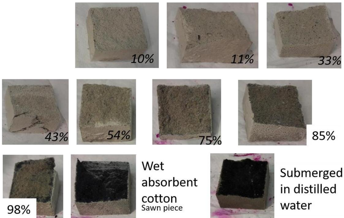
Figure 3-12: Oxidation at 20°C for foamed concrete after 1000 days exposure to a relative humidity of cubical samples with an edge of 5 cm
