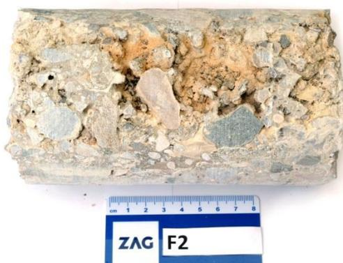
Figure 4-14: A sample from the Fala hydroelectric power plant (a core with entrapped air)
