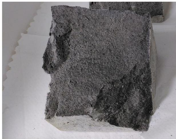
Figure 3-15: ‘Oxidation’ at around room temperature after exposure to the saline solution in Table 3-5 for foamed concrete with CEM I of a cubical specimen with an edge of 10 cm
