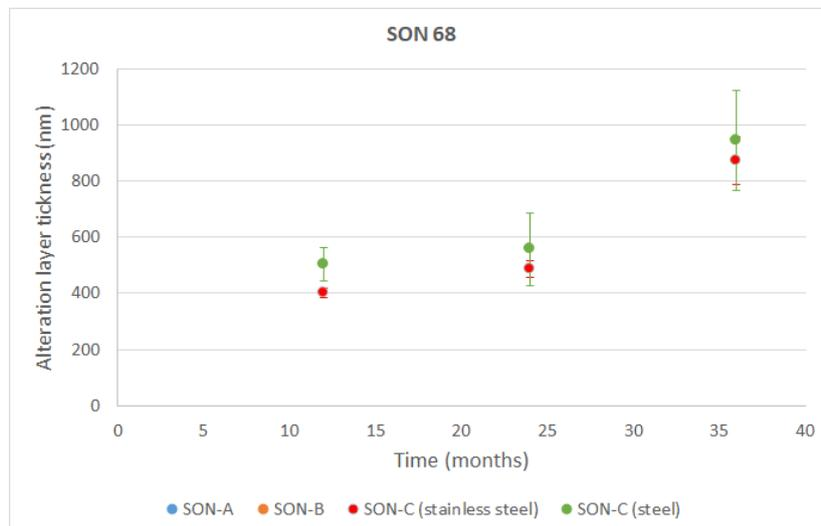
Figure 4-6 – Alteration layer thickness measured on SON 68 glass after 6, 12, 24 and 36 months. Steel canister (A), steel canister coated with magnetite (B) and “Sandwich” (C).
