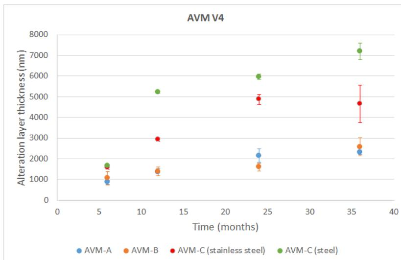
Figure 4-4 – Alteration layer thickness measured on AVM glass after 6, 12, 24 and 36 months. Steel canister (A), steel canister coated with magnetite (B) and “Sandwich” (C).
