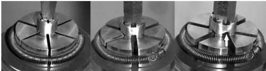
Figure 1: Stages of sample deformation during the test: Small elastic deformation (left); large plastic deformation, the width and wall thickness of the ring is visibly reduced (middle); ductile crack nucleation just before failure at the centre of a region affected by significant necking (right).
