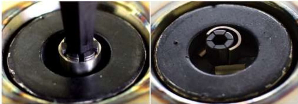
Figure 2: State of a ductile (627 ppm hydrogen, left side) and a brittle (2059 ppm hydrogen, right side) hydrogenated E110opt sample after the same spike displacement.
