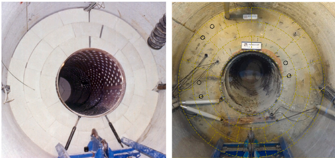
Fig. 2. Appearance of the bentonite barrier around Heater #2 during installation in 1997 and during dismantling in 2015 (the block contours were difficult to tell apart and have been indicated by discontinuous lines.) Examples of the location of samples drilled for gas testing are marked with circles.
