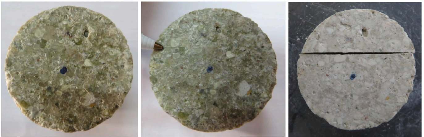
Fig. 7. Appearance of sample BC-53-2 before (left) and after (middle) gas testing. The interface split only after drying in the oven (right).
