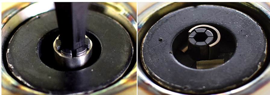
Fig. 9. State of a ductile (EoH4 627 ppm hydrogen, left side) and a brittle (EoH8 2059 ppm hydrogen) hydrogenated E110opt sample after the same spike displacement.
