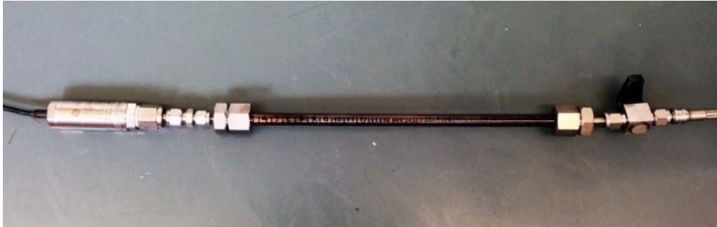
Figure 5. Gas tight specimen assembly connected to pressure gauge and with attached pressure transducer, ready for mechanical testing.
