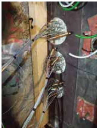
Three cable flanges, which carry in total 51 sensor wires, photographed from inside (left) and outside (right) plug section 2
