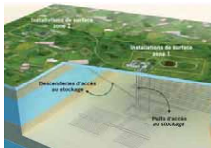
Disposal facility of Cigéo project in France (Labalette et al., 2013)
